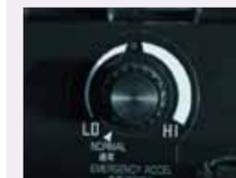
If unexpected trouble is experienced with the ITCS mechatronic control system, the machine can still be operated using the emergency acceleration system. Digging modes are also automatically relayed to an emergency system so that digging can continue with minimum down time.
