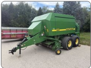
Lot 59 John Deere 100 Large Square Baler, PTO Driven, Tandem Axle Flotation Tires, approx. 72" pickup, Power-Feed feeding system, 1000 PTO, hydraulic pickup lift, tandem axle, rear bale chute, light kit, tandem flotation tires
